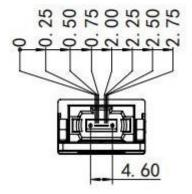
Attention: To minimize MPO connection induced reflections, an MPO receptacle with 8-degree angled end-face is utilized for this product. A male MPO connector with 8-degree end-face should be used with this product as illustrated in Figure below.
